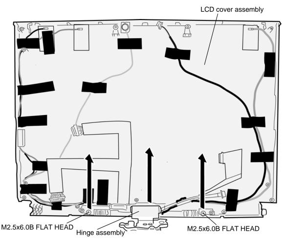
Figure 4-58 Removing the wireless LAN antenna/Internal microphone/web camera cable
